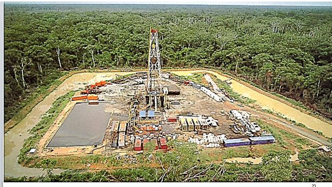
Fig. 9. A land drilling rig
