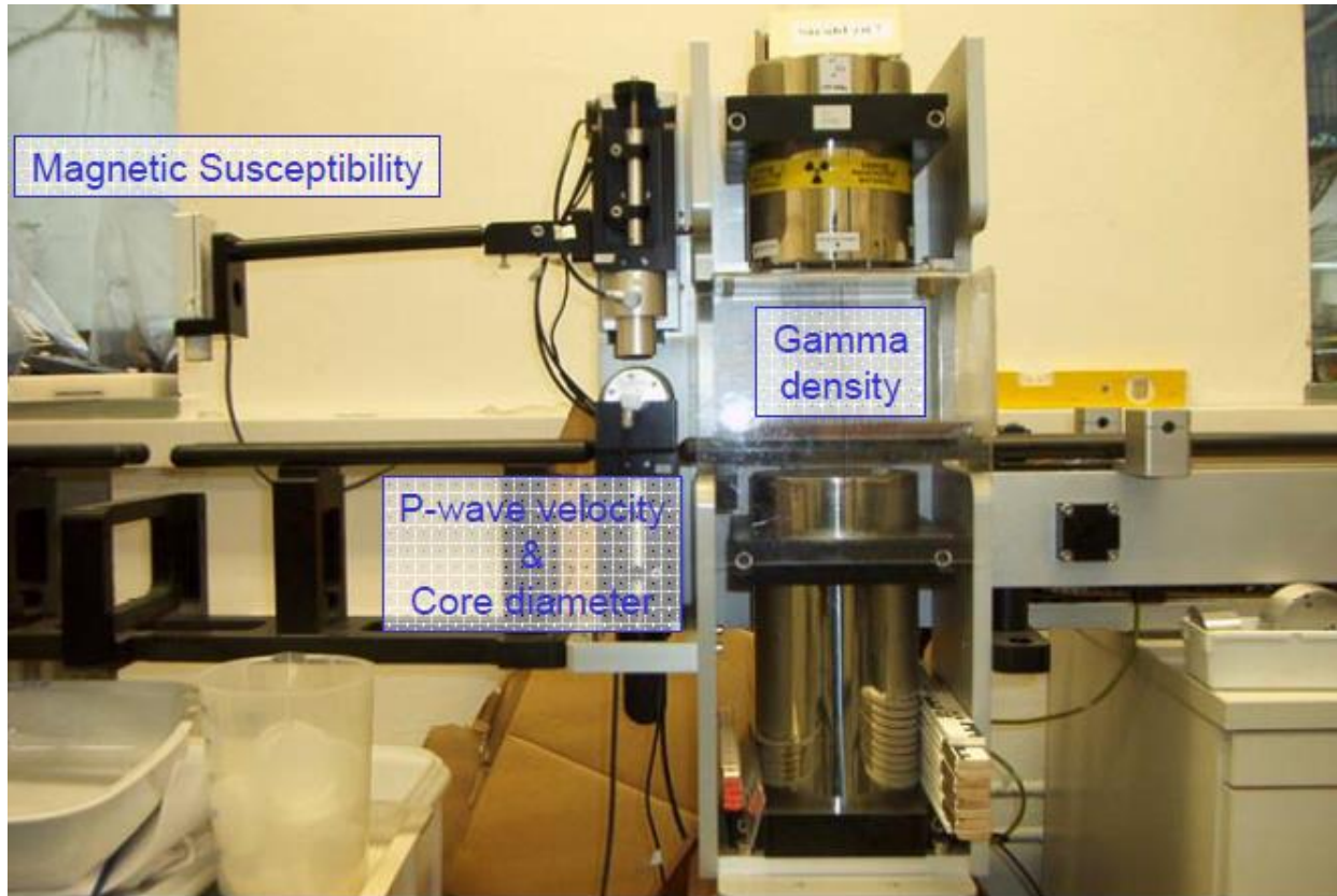
Figure 4: Actual laboratory picture of the MSCL logger
